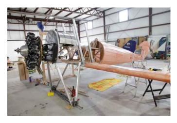
Major tasks remaining include all wiring, piping and cooling air baffling for the engine (including the fuel and oil system), reception and installation of prop, instrument
