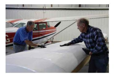
Below is the aircraft as it is at the time of this newsletter. All surfaces are covered, and all surfaces are sealed but the top wing. Sheet metal work on the forward fuselage is in process, but was removed when this photo was taken after remounting of the bottom wing.
